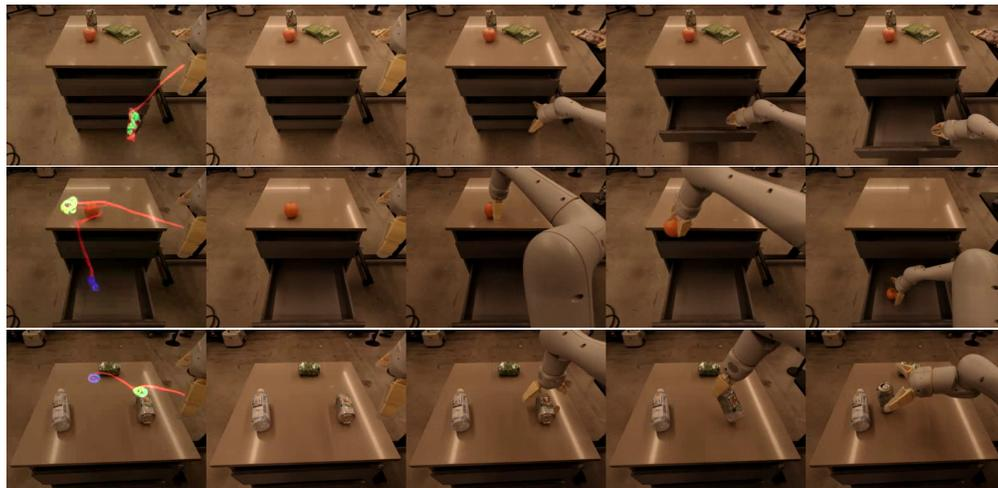
Figure 16: Example trajectories from image generation models. Each row shows the trajectory sketch overlaid on the first frame and the rollout. The language instructions are: open middle drawer, place orange into middle drawer, move 7up can near blue plastic bottle.
