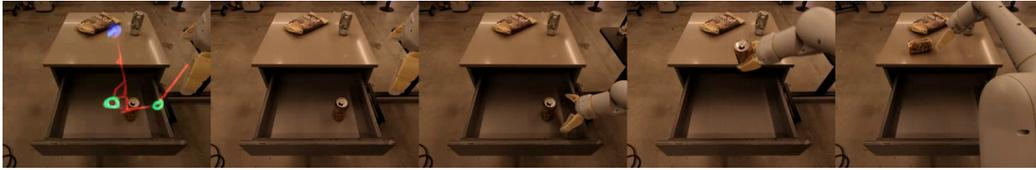
Figure 7: Example trajectory from image generation models. From left to right, the first image shows the overlaid trajectory sketch, and the next 4 images show the rollout conditioned on it. The language instruction is: pick orange can from top drawer and place on counter.
