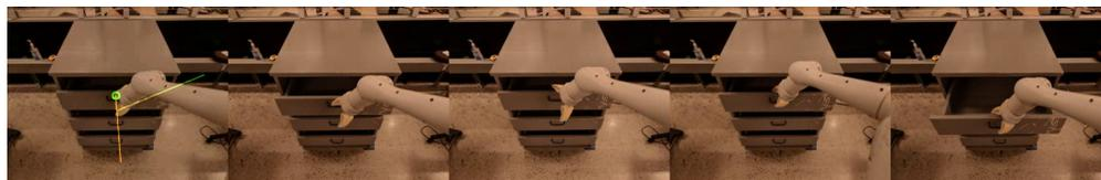
Figure 20: Example of retry behavior. The first image is the trajectory sketch generated from the CaP overlaid on the initial observation. The remaining images show the rollout. The robot first attempts to open the drawer by grasping its handle, but fails (2nd image). Then, it retries to open the drawer by grasping the edge instead.
